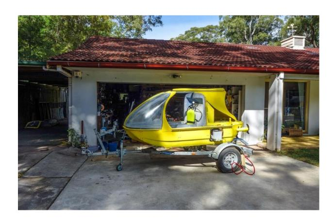
It took the most time for us to restore the frame and the hull. Rust damaged the frame in some places so we had to weld strengthening somewhere. The cladding and plastic windows were not in very good condition either and we had to tinker with them and even make something anew. However, day after day we did our work and one day all the work was done.
